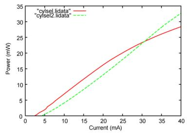
Difference in L-I is mainly due to current spreading effect.
