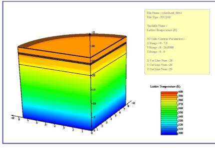
Thermal VCSEL simulation: temperature distribution
