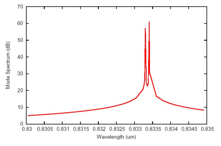
Different lateral modes produce different propagation constants which causes multiple peaks in simulated emission spectrum as a result of the self-consistent calculation.
