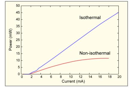
L-I characteristic: Iso- vs. Non-isothermal simulation
