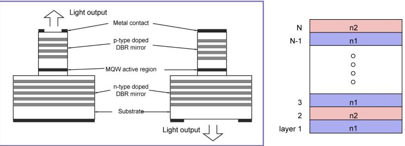
Schematic of surface emitting lasers of front and back emission.
