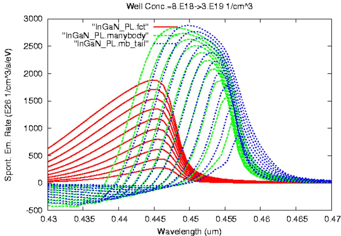
Many-body simulation shows that spontaneous emission peak blue shifts with carrier density, not seen in free-carrier theory
