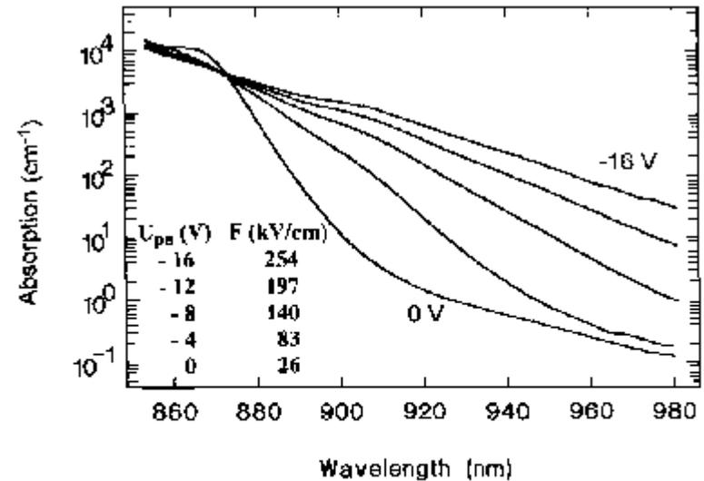
Fig. 1. Spectral dependence of the absorption coefficient  $\alpha(\lambda)$  of the p-i-n DHS for a set of various voltages  $U_{pn}$  which are shown together with the corresponding electric fields in the intrinsic region.
