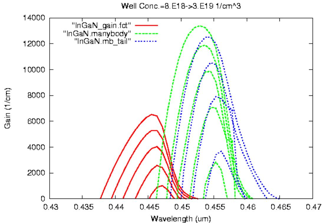
InGaN results show strong Coulomb enhancement (by a factor of 2) in the spectra and band-gap reduction. 1s exciton binding energy is about 46meV in good agreement with Chow's calculation.
