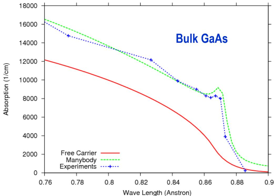
Free-carrier theory underestimates absorption, especially near the band edge. Manybody Coulomb enhancement based on the pade approximation gives accurate results compared with experiments.
