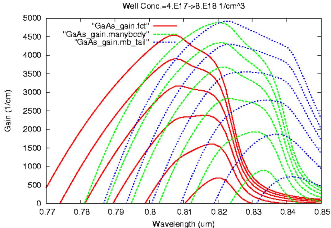
Coulomb enhancement (about 10%-20%) is not so strong for GaAs at high carrier density, but band-gap renormalization reduces the band-gap.
