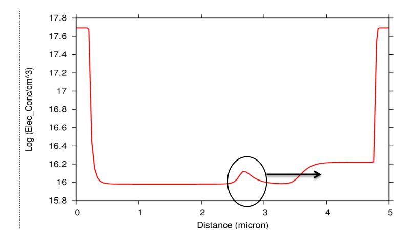
• Initial voltage pulse introduces an accumulation region (n>n<sub>0</sub>) which propagates towards the anode in order to accommodate the new voltage bias.
