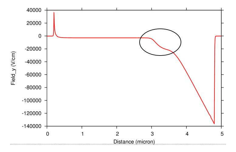
• Field perturbation from voltage pulsed "merged" into existing high-field region: no formation of separate field domains.
