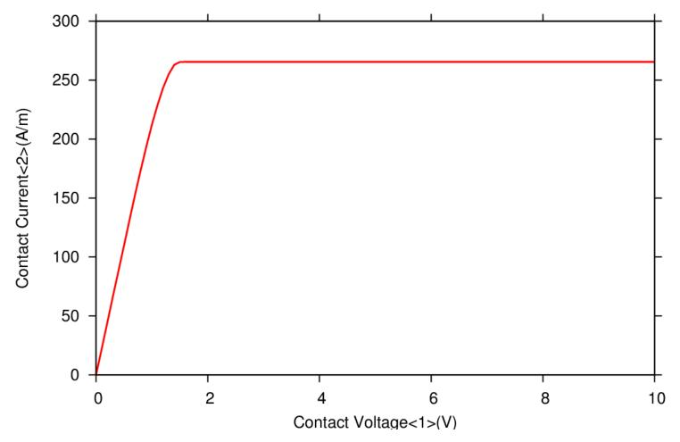
• From Drift-Diffusion model, no pulsations can be observed under steadystate conditions (all  $\frac{d}{dt}$  terms are zero)
