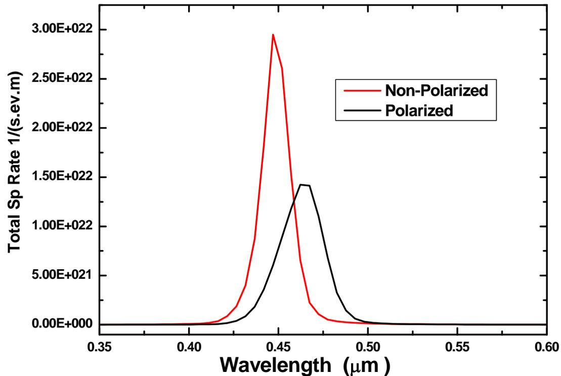
Polarization field decreases the interband recombination rate and results in the red shift of luminous energy .
