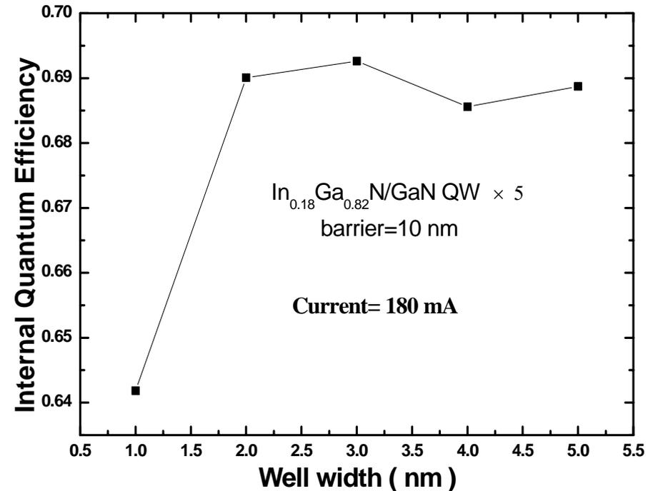
For the well with 1nm thickness, polarization charges make larger effects than the other four cases.
