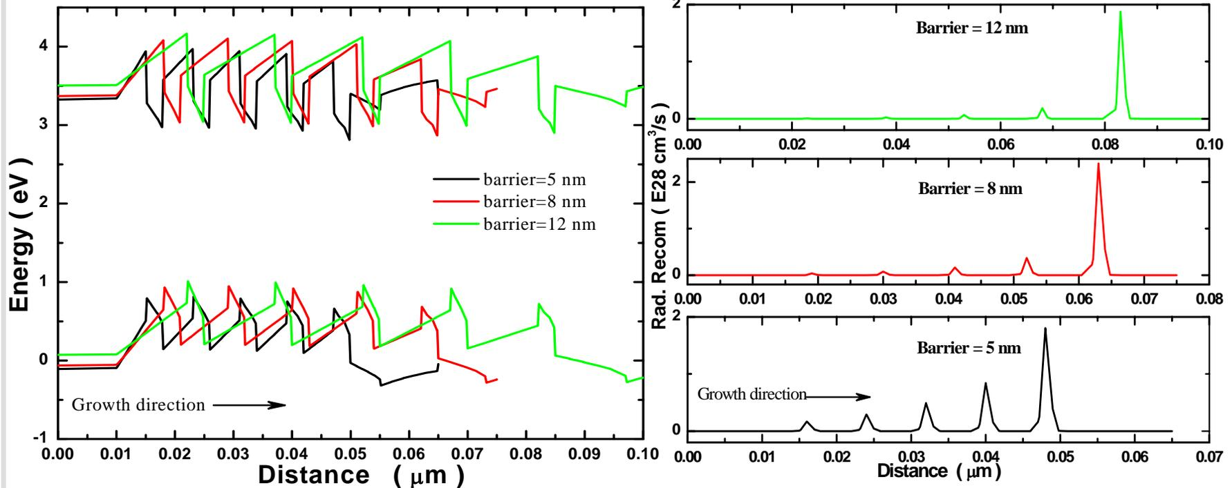
Thinner barrier makes holes easier to diffuse from p-region to MQW region, which totally increases radiative recombination rate
