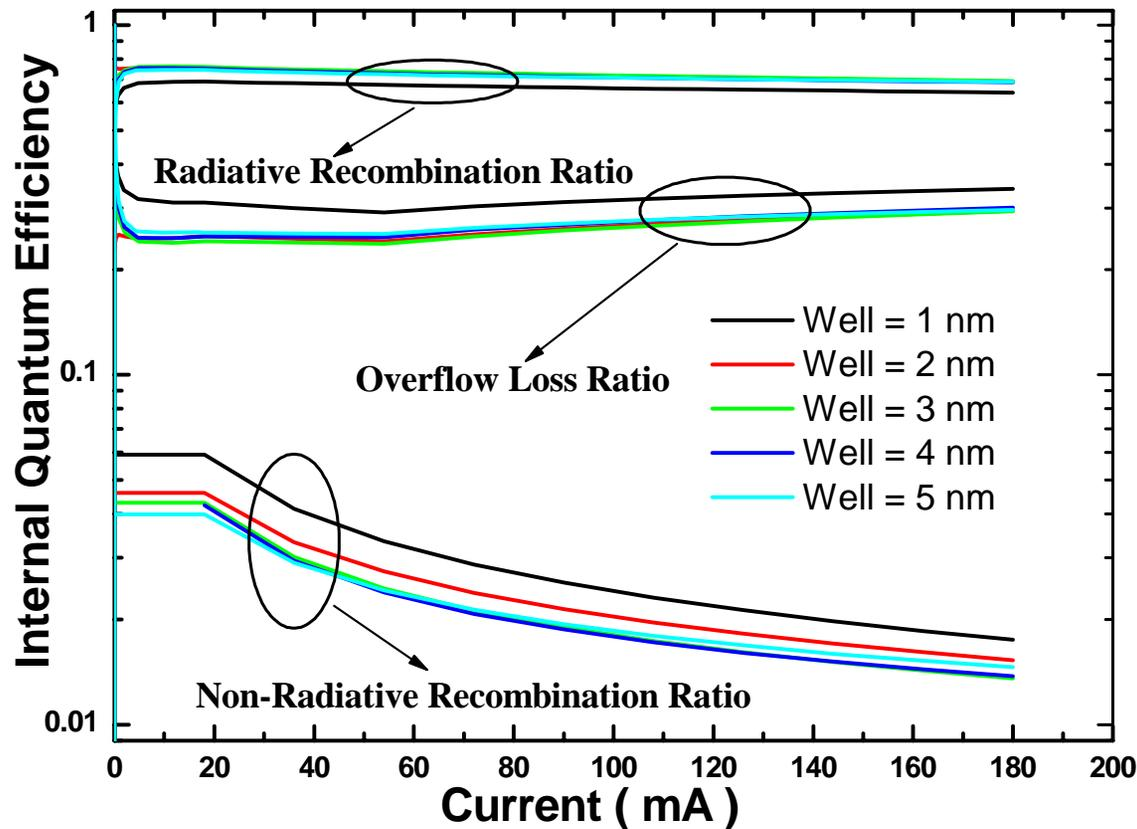
With increase of well width, the overflow loss decreases because the quantized levels are closer to the well bottom, making overflow less likely.
