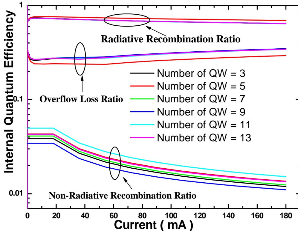
Overflow loss plays an important role on polarized-LED IQE, which proves the conclusion in the former page.
