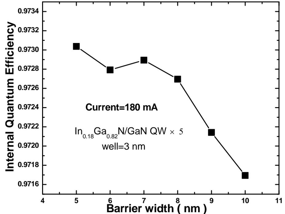
Narrow barrier are beneficial to get higher efficiency for InGaN/GaN MQW LEDs when there are no polarization charges.
