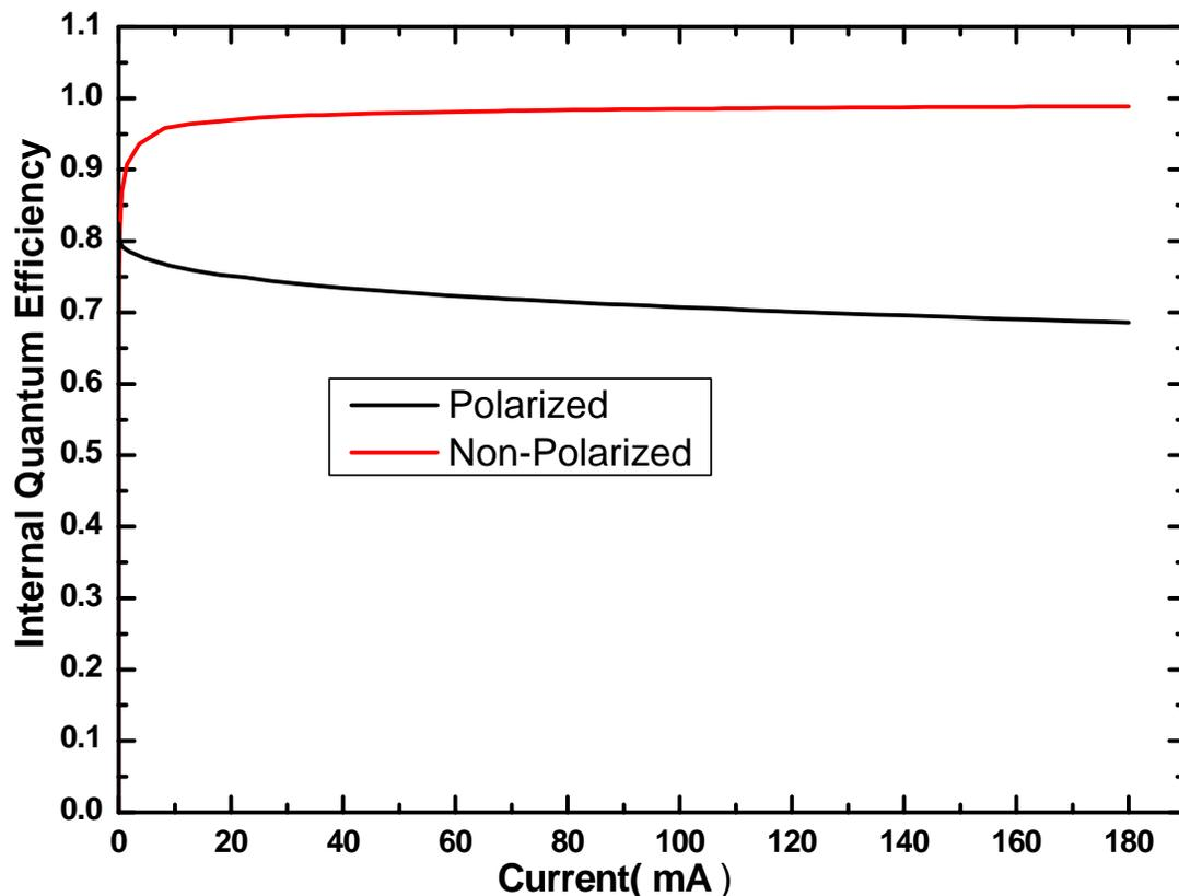
Polarization charge in the MQW structure plays an important role leading to the low luminous efficiency of InGaN/GaN MQW LEDs.
