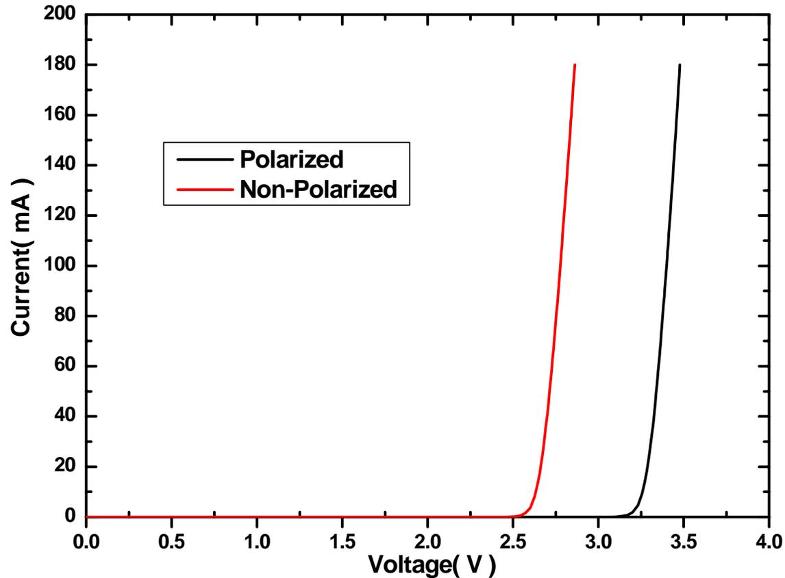
Polarization field increases the threshold voltage of LED.
