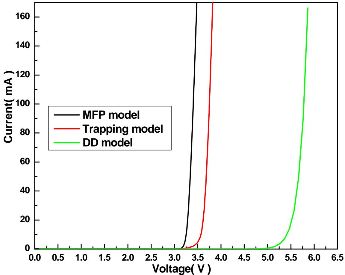
Drift-diffusion model shows unrealistically high turn-on voltage
