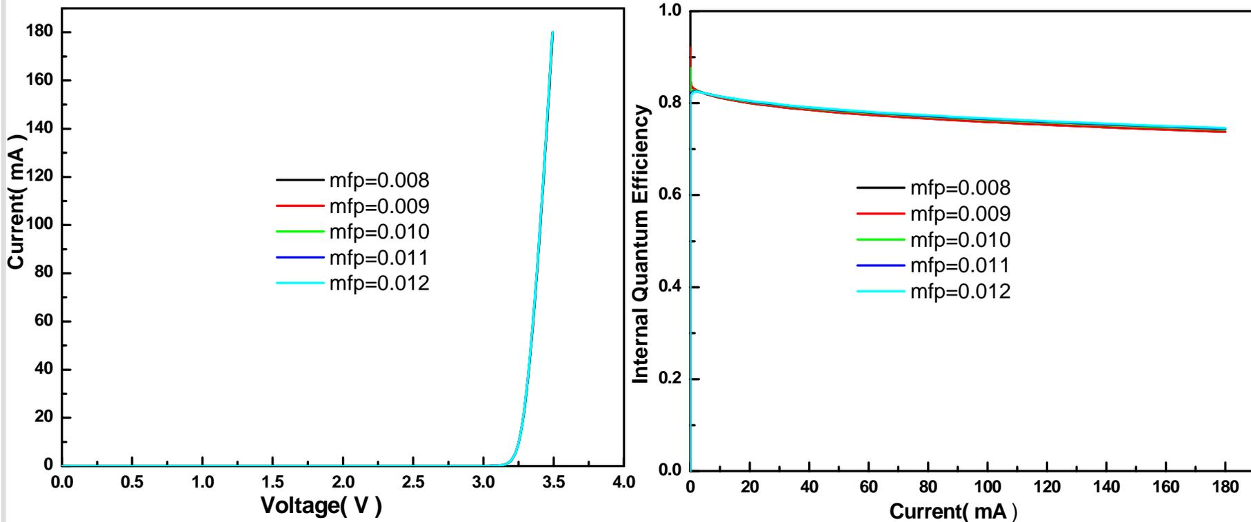
In MFP model, **mfp** is used for the exponential factor to control the non-local current flow intensity. In Crosslight, the default value is 0.01 ( $\mu\text{m}$ ).
