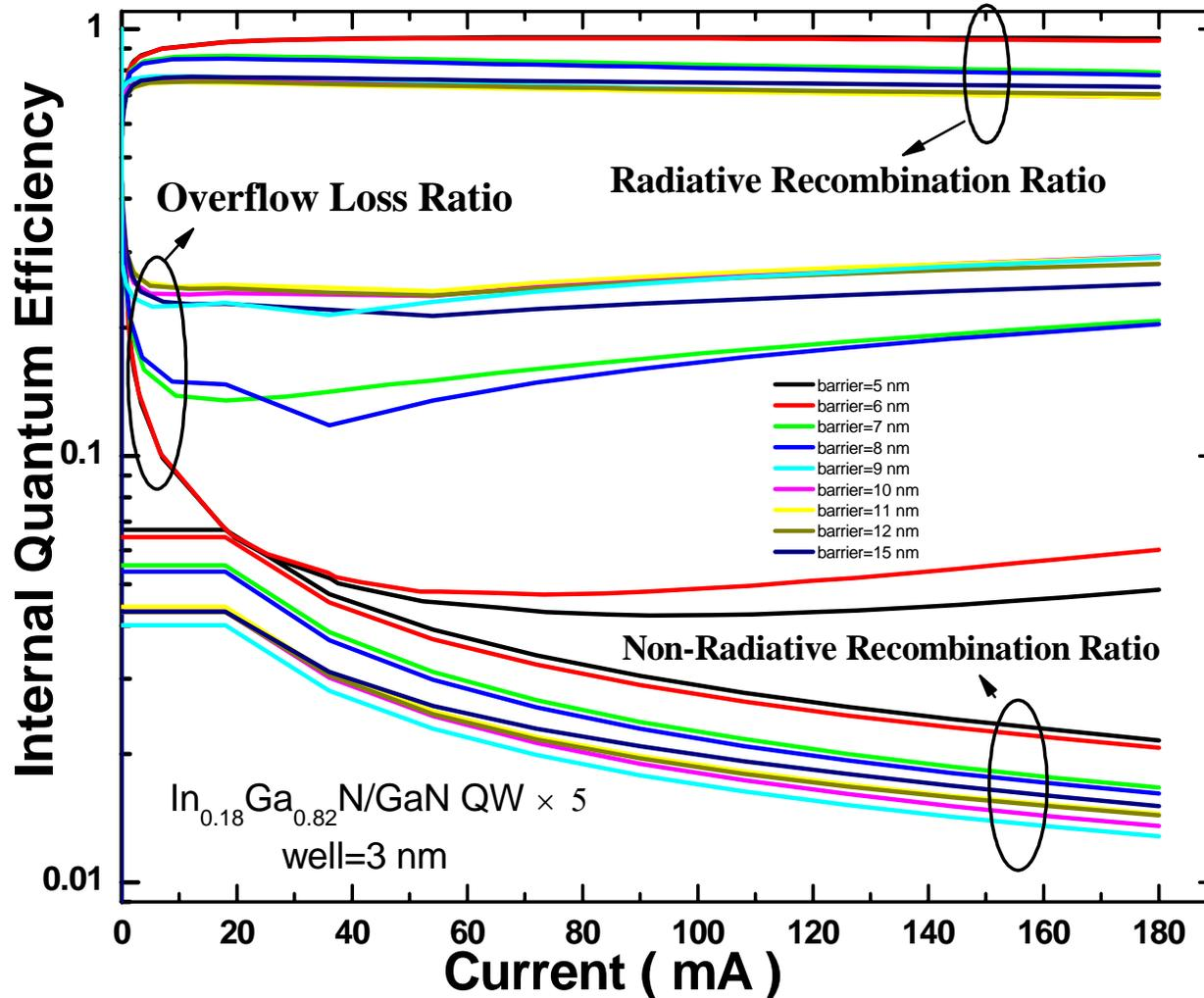
Overflow loss is responsible for the dependence of efficiency on the width of barrier.
