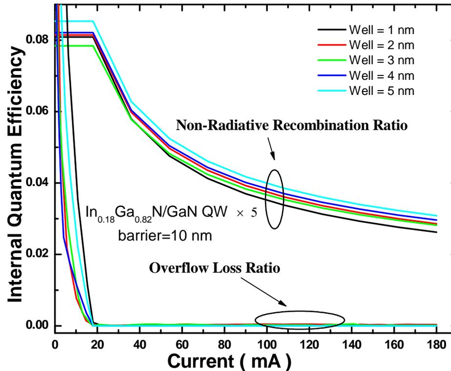
Non-radiative recombination decreases with increase of well width and overflow loss is almost zero.
