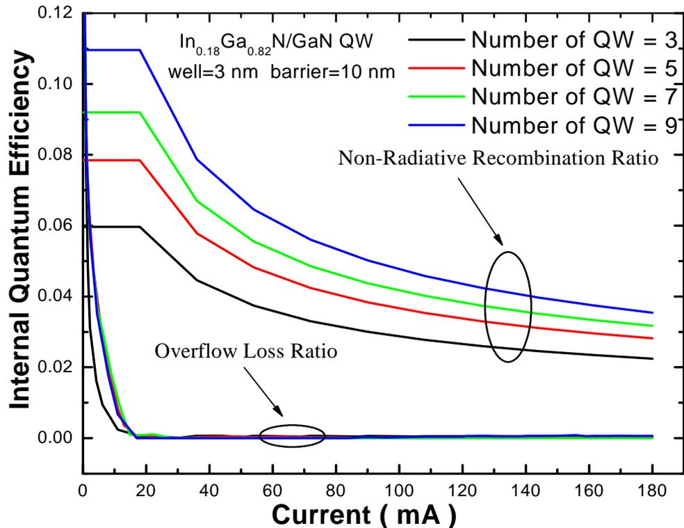
Increase of non-radiative recombination are responsible for the slight decrease of IQE with increase of QWs in InGaN/GaN MQW LEDs with no polarization charges where overflow loss is very small.
