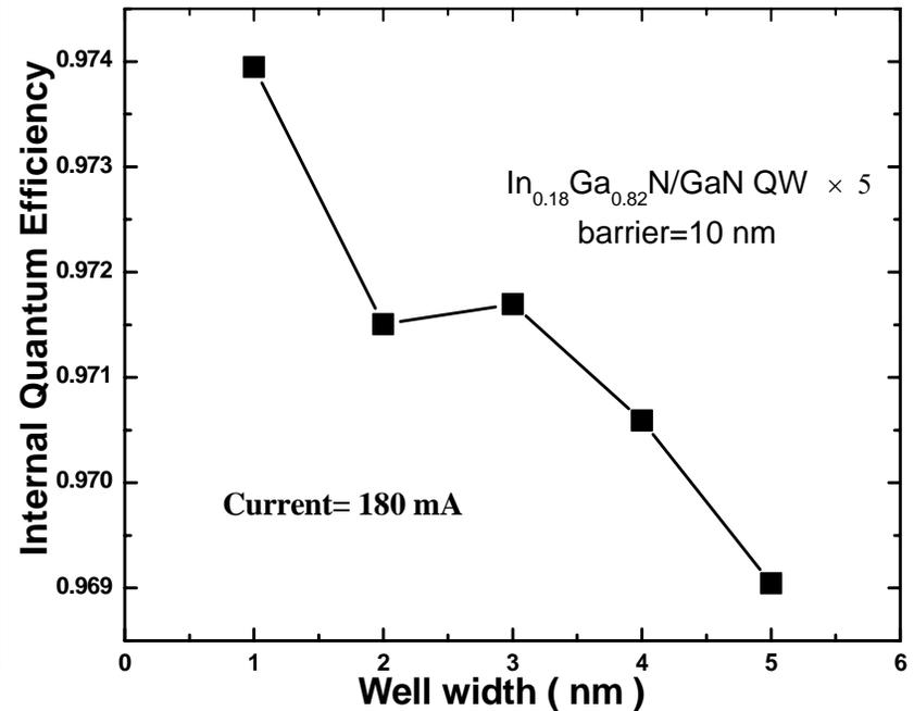
IQE has weak dependence on the well width with the polarized counterpart
