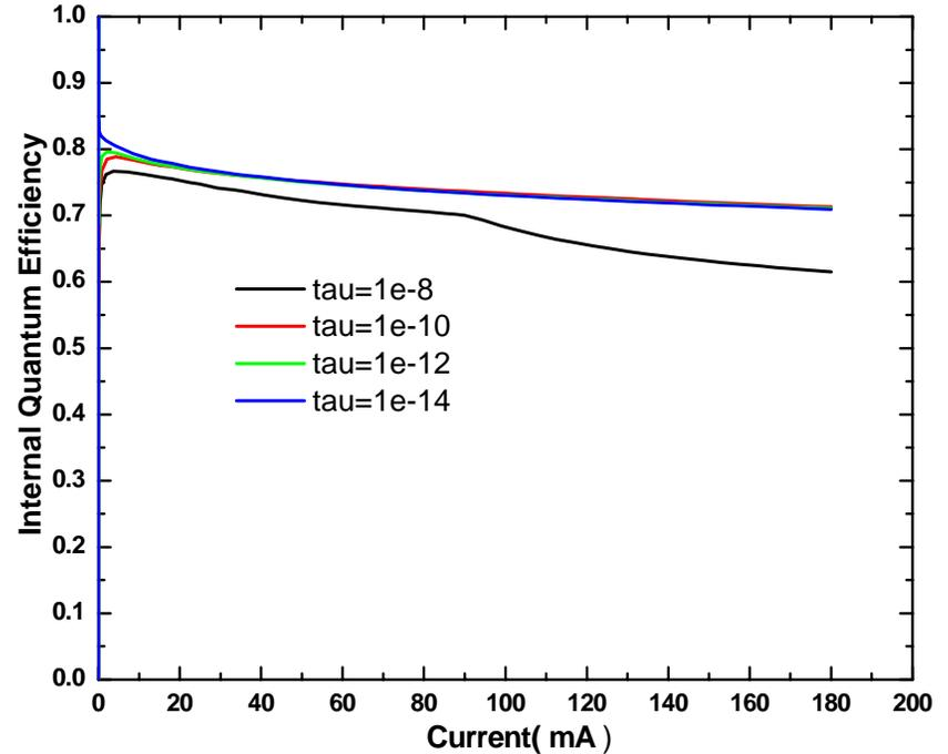
**q\_trap\_tau** is the time constant for the 2-Fermi level trapping model.
