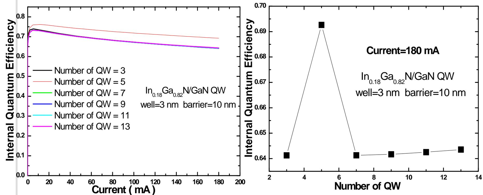
For integrated effect on LED IQE, QW number = 5 shows an optimal situation
