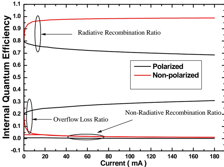
More overflow loss of current is generated by Polarization charge leading to the drop of efficiency at high current, which is in good agreement with the results as shown in Ref. Appl.Phys.Lett. 91,183507.
