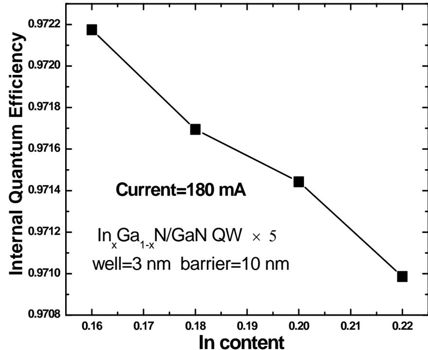
The  $\text{InGaN}/\text{GaN}$  MQW LEDs have similar properties with the polarized counterpart, but the IQE is less sensitive to the indium composition.
