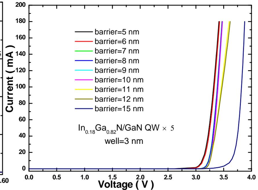
The thicker barrier is, the higher threshold voltage is.
