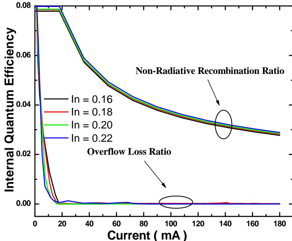
IQE in InGaN/GaN MQW LEDs without polarization effects is affected heavily by non-radiative recombination instead of overflow loss.
