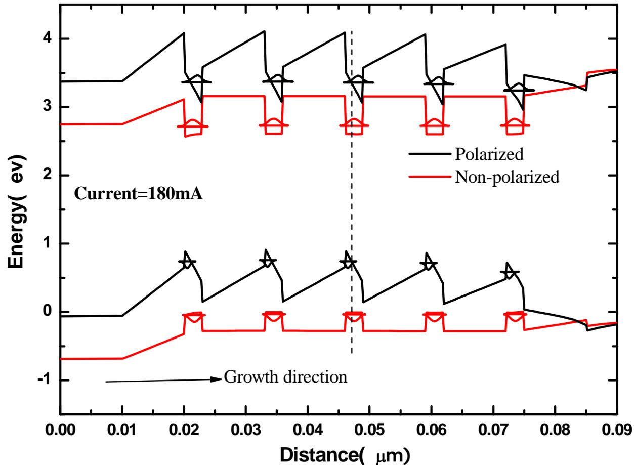
Polarization field tilts the energy band and induces the spatial separation of the electron and hole wave functions.
