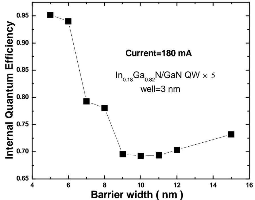
Width of barrier has important effect on the efficiency of LEDs.
