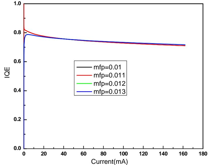
**mfp** is the electron or hole mean free path. In the trapping model, it controls the transport of carriers that fly-over and are not trapped. In Crosslight, the default value is 0.01 ( $\mu\text{m}$ ).
